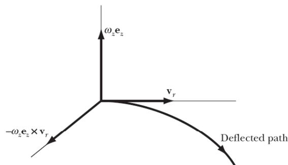
**Figure 8-4** – In the Northern hemisphere, a particle projected in a horizontal plane will be directed to the right of its motion. The opposite will happen in the Southern Hemisphere.
