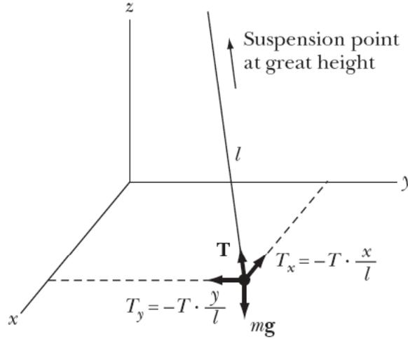
**Figure 8-7** – Geometry of Foucault’s pendulum. The acceleration vector is along the  $-z$ -axis, and the tension  $\mathbf{T}$  is broken down into components along the  $x$ -,  $y$ -, and  $z$ -axes.
