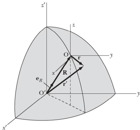
**Figure 8-3** – The inertial reference system  $x'y'z'$  has its origin  $O'$  at the centre of the Earth, and the moving frame  $xyz$  has its centre near the Earth's surface. The vector  $\mathbf{R}$  gives the Earth's radius.
