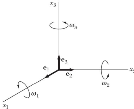
**Figure 8-2** – With this definition for the set of axes, and with  $\omega_i = d\theta_i/dt$ , for  $i = 1, 2$ , and  $3$ , we can determine the effect of the rotations on the different basis vectors.
