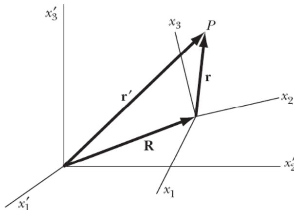
**Figure 8-1** – The  $x'_i$ 's are coordinates in the fixed system, and  $x_i$  are coordinates in the rotating system. The vector  $\mathbf{R}$  locates the origin of the rotating system in the fixed system.
