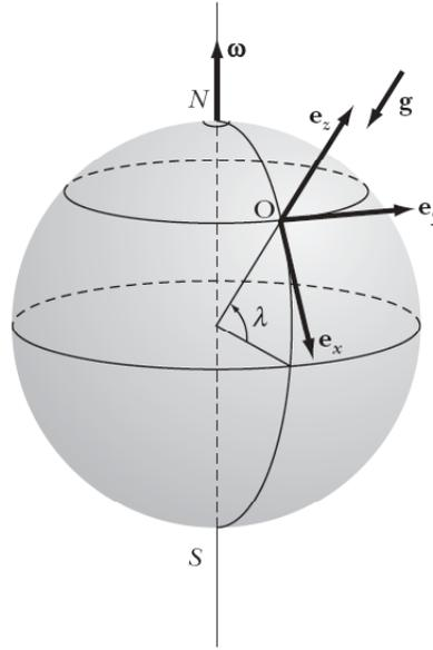
**Figure 8-6** – The coordinated system “attached” to the Earth’s surface, for finding the horizontal deflection of a free-falling particle. The  $\mathbf{e}_x$  and  $\mathbf{e}_y$  bases vectors are, respectively, in the southerly and easterly direction.
